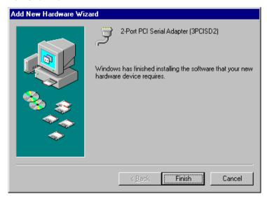
11. Click **Finish** to begin the second part of the driver installation which installs the Com port driver for Port A & B.
